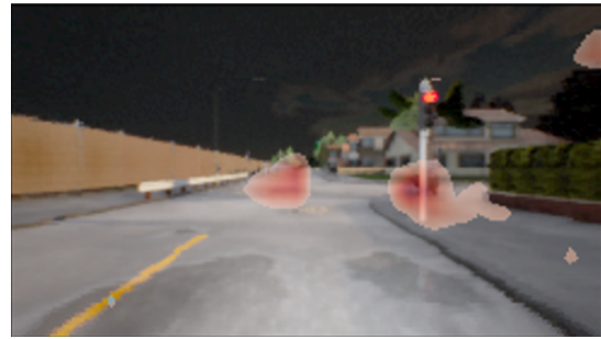
Fig. 2: Saliency map generated by using blur-based saliency (Sec. III-A) for LbC model [18] at instant a vehicle comes to a stop after which it fails to restart. The bulk of saliency weight is at the traffic light’s base — a non-causal region which indicates causal misattribution.
