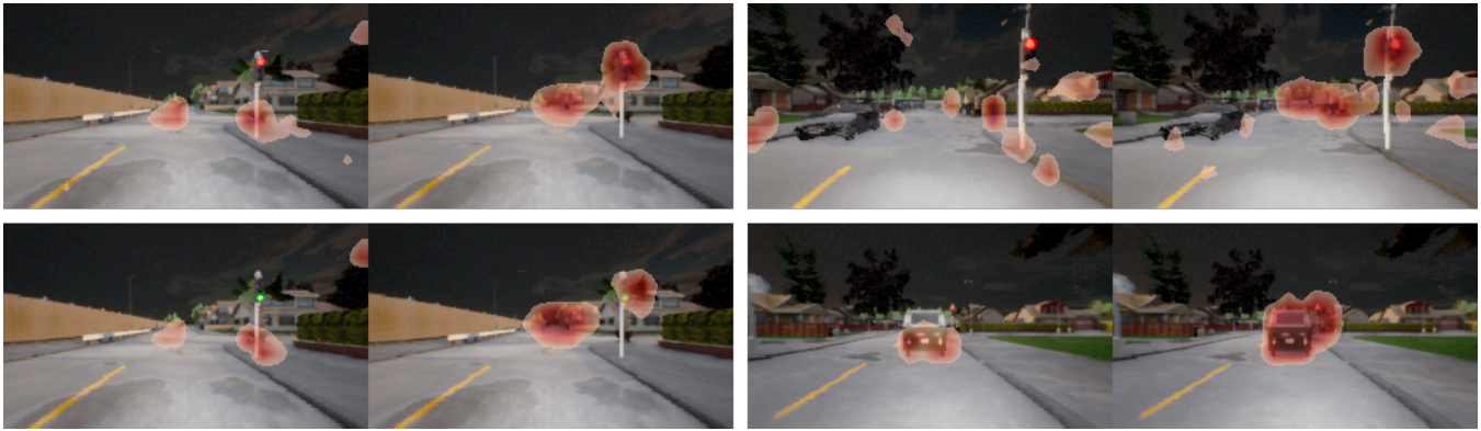
Fig. 7: Model saliency example pairs (Sec. III-A) showing LBC model saliency before and after gaze-based supervision. Within each pair, left images correspond to the pre-trained model with no gaze-based training and right images correspond to our model fine-tuned on the “Mix” dataset with gaze and control supervision. Overall, the gaze supervised model’s saliency lies more on causal scene elements such as traffic lights and the space in front of the vehicle.
