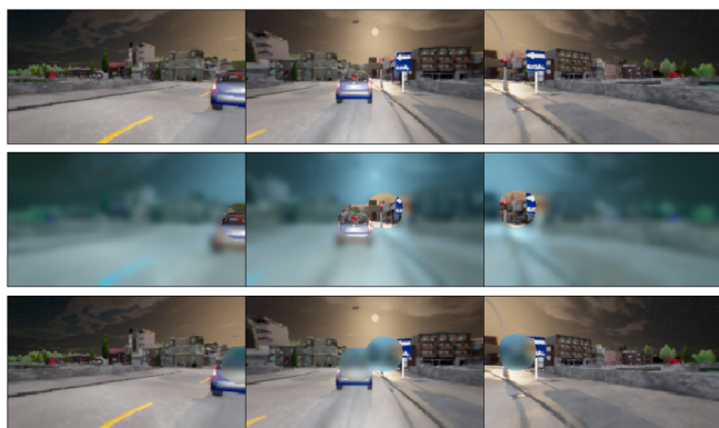
Fig. 6: Example triplet in more detail with gaze-contingent blur applied. In order (top-bottom): Anchor inputs (no blur), Positive image (blur in non-attention regions), Negative image (blur in attention regions). Blue shading is added to illustrate the blurred region (not present in training input).
