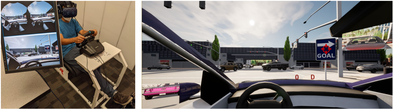
(a) Physical setup with participant driver in driving pose, alongside experimenter's setup monitoring the simulation. (b) First person DReyeVR simulator perspective during the same episode with eye reticle (red crosshair) denoting eye gaze on in-world navigational sign that gives drivers route direction. The crosshair is only for illustration (not shown in VR).
