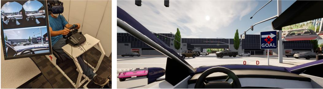
(a) Physical setup with participant driver in driving pose, alongside experimenter’s setup monitoring the simulation.
